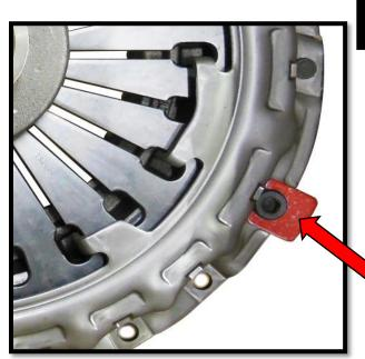
The strap locating bolts remain torqued and are NOT removed
