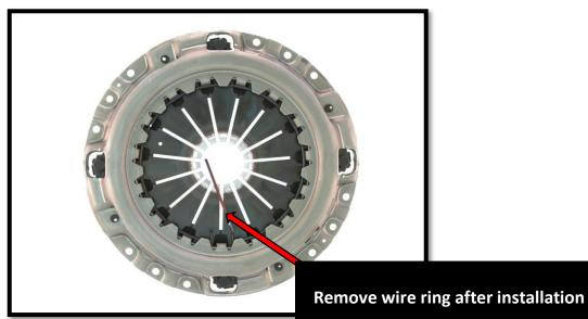
Hold Down Plates need be removed "AFTER" clutch is installed to the flywheel and "BEFORE" installing gearbox. Failure to remove these plates will result in clutch slippage and likely damage to the clutch assembly and/or transmission.
